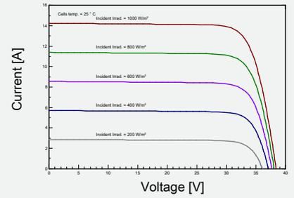
**P-V CURVES OF PV MODULE(430W)**
